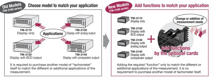
As measurement becomes more diverse, it is not easy to select a suitable model that meets your application. Measuring requirements are often changed or added. The TM-3100 series enables you to respond instantly to changes in these diverse needs by adding functions to match the application.
