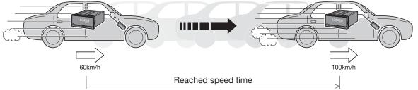
Display the acceleration, which is calculated at every 1 second interval.
