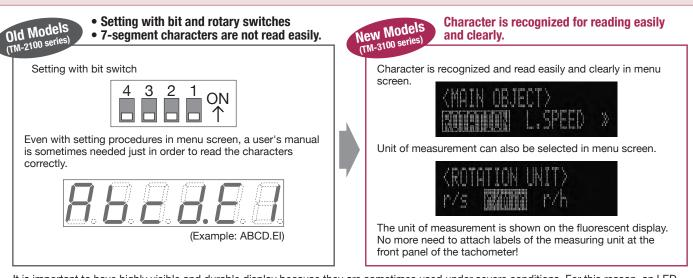
It is important to have highly visible and durable display because they are sometimes used under severe conditions. For this reason, an LED display is normally used. There are limitations, however, of the character that LEDs can display, causing unreadable character and other problems. The TM-3100 series uses a fluorescent display tube, maintaining durability while greatly improving readability.
